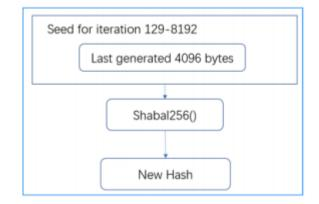
Generate a final hash (Final Hash), use the 8192 hashes generated to create a final hash. All 8192 hash values and the first 16 bytes are used as seeds, and the final hash is generated after the Shabal256 function is calculated.
