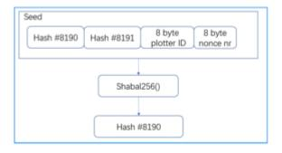
Create a new hash. For all 8192 hashes, continue to append the hashes to generate a new seed. After 128 iterations, the seed length exceeds 4096 bytes. For the remaining iterations, only the last 4096 bytes are read.
