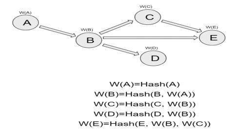
The prover needs to store the W value of each node for the verifier to select and check during the verification phase randomly. The interaction process between the prover and the verifier is as follows:
