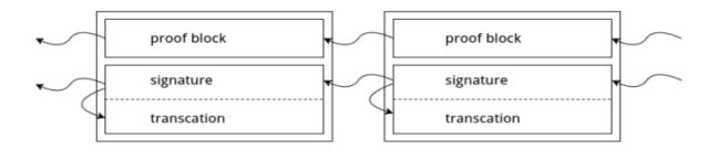
This chain contains two parts, the consensus proof sub-chain and the signature sub-chain, and the signature sub-chain also contains the corresponding transaction information.
