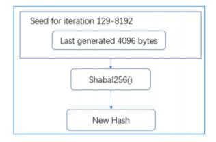
Generate a final hash (Final Hash), use the 8192 hashes generated to create a final hash. All 8192 hash values and the first 16 bytes are used as seeds, and the final hash is generated after the Shabal256 function is calculated.
