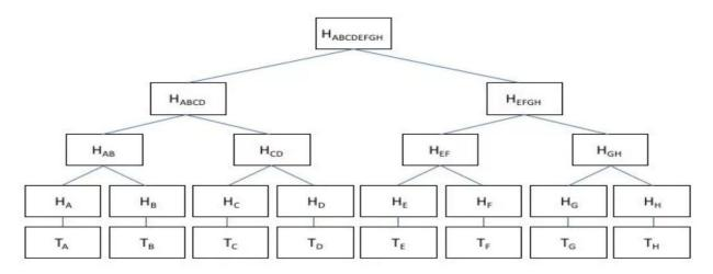
The prover uses the W value of each node as the leaf node of the Merkle tree, calculates the root of the Merkle tree as one of the parameters, and sends it to the verifier in the initial phase. In the verification phase, the verifier only needs to verify the value of a certain node whether the value of W exists in the Merkle tree sent in the initial stage of the first step.
